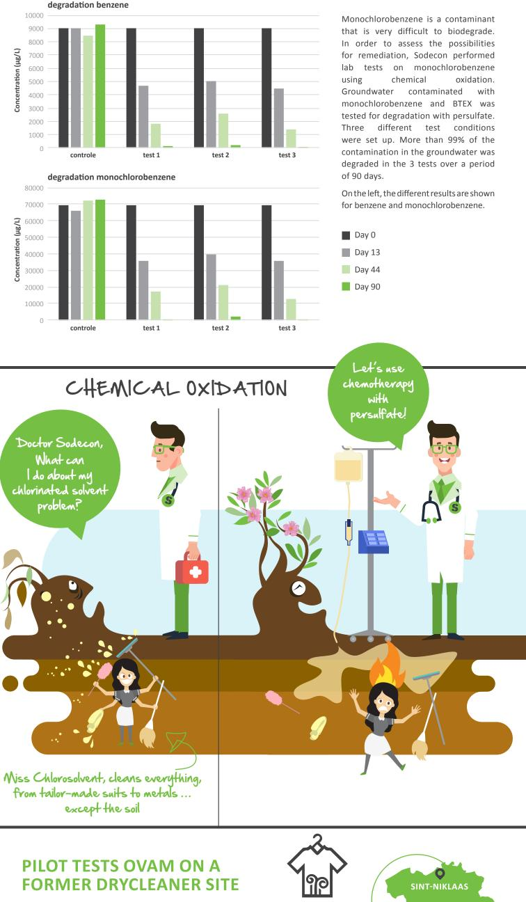
By commission of the OVAM (Flemish Public Waste Agency), we are performing laboratory and pilot tests for the remediation of a dry cleaner site in Sint-Niklaas. On the one hand, a test with chemical oxidation using persulfate and, on the other hand, a test with biological and chemical reduction using a mixture of zero-valent iron and a long-lasting carbon source will be performed. The results of the tests will be used to remediate the contamination on the site so that it can be redeveloped.
